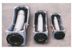
The composite hose is secured within two reinforced steel side plates (primed or galvanized carbon steel or stainless steel). These side plates are joined by a stainless steel pivotal pin that uses stainless steel bushings and spacers to eliminate binding and assure flexibility.
