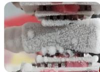
3 After the test temperature is reached, the system will start the stabilization time, ranging from 15 to 500 minutes.
