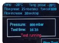
5 If the system recognizes a rapid pressure decrease, the system will store the maximum pressure value as the test result.
