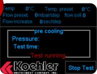
4 Once the test begins, the instrument will begin applying pressure on the grease in the test nozzle in incremental steps of 30 seconds.
