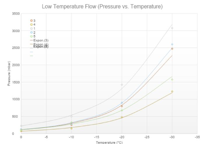
The K95300 exhibits a high level of reliability and accuracy, all in accordance with the standardized Kesternich Method. With the K95300 being able to report a high quality of results in a very efficient manner, it would be justified to conclude that this instrument is one of the best choices available for determining the lubricating greases that are most suitable for low temperature operating conditions and applications.
