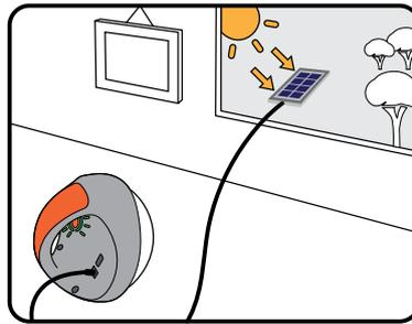
2. Keep lamp Indoors while charging. Plug panel into the lamp.
