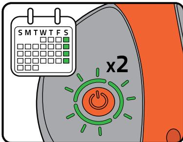
4. Fully charge the battery when first purchased and at least once per week. LEDs will double flash every 10 seconds when fully charged.
