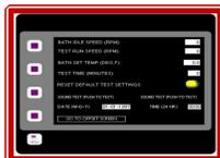
1 Prior to running a test, check all the testing setting. The default setting is for ASTM D7548 method or use custom parameters.
