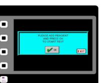
3 After pour 50 mL of sample into the test jar and start the test, the sample will be stirred at 900 RPM for 1 hour under default.
