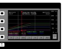
4 Once the test begins, the instrument will increase both bath and sample temperatures with certain amount of time to the desirable temperature.
