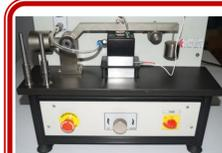
1 The parts of the K94190 instrument should be assemble according to the instructions on the operation manual. 50 mL of fuel is added into the fuel bath.
