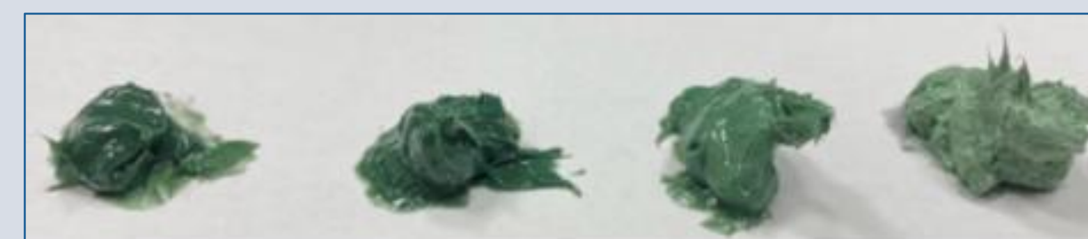
Figure 2: Grease with 0% water (left), 1% water (middle left), 10% water (middle right), and 50% water (right).
