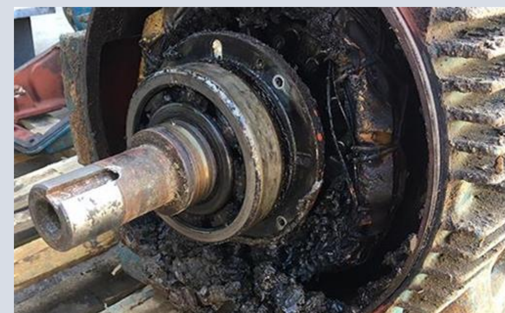
Figure 1: Machine Featuring Severe Weather Damage.
